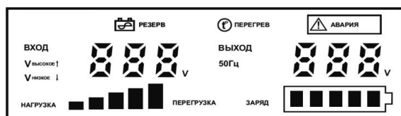
Рисунок 3.1 — Светодиодный графический индикатор изделий SKAT-UPS 100T, SKAT-UPS 300T, SKAT-UPS 500T, SKAT-UPS 800T, SKAT-UPS 1000T, SKAT-UPS 2000T, SKAT-UPS 2500T, SKAT-UPS 3500T, SKAT-UPS 5000T
